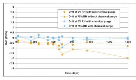
*Figure 4*: Sensor drift with and without chemical purge measured in a wood drying process. Test period of 3 years.
