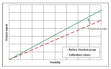
Figure 2. Sensor performance is restored by chemical purge.
